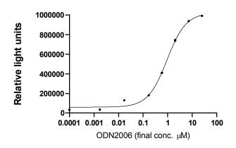
Figure 1. Example of ODN2006 calibration curve.
