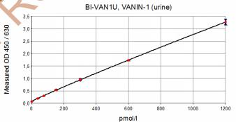
The quality control (QC) protocol supplied with the kit shows the results of the final release QC for each kit lot. Data for OD obtained by customers may differ due to various influences and/or due to the normal decrease of signal intensity during shelf life. However, this does not affect validity of results as long as an OD of 1.50 or more is obtained for the STD with the highest concentration and the values of the CTRLs are in range (target ranges see labels).
